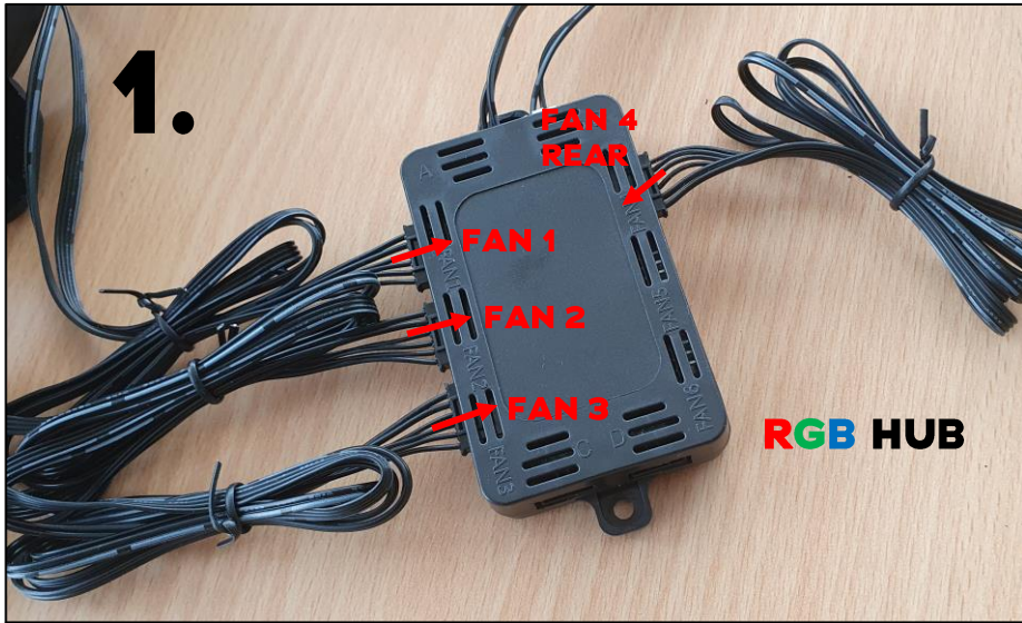
1. Connect fan cables to RGB HUB accordingly. Numbers are visible on the HUB for assistants.
